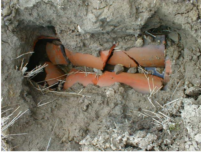
Figure 4. Damaged drainage tile can result in saturated soil and standing water upstream from the blockage.
